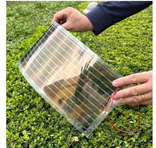
Organic photovoltaic modules (2.5W)
