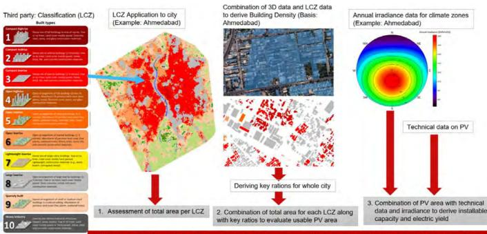
BIPV potential - 6.7% of façade area would be used to estimate the potential for BIPV of future building stock (33% of total facade area is considered based on +/-60 degrees around south, out of which only 20% area is used)
