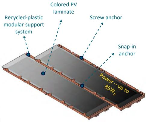
The waterproofing in ensured by the overlapping both of laminates, which create a main water flow plane, and of modular plastic elements, which constitute the waterproofing layer.
